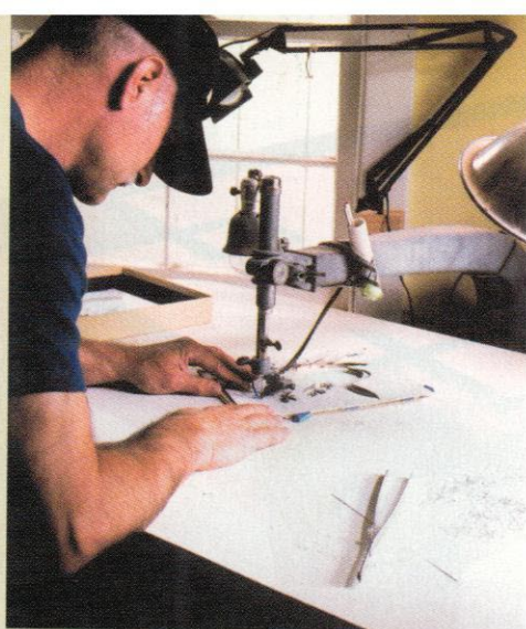
To cut the pieces for his designs, Schürch uses a technique called packet cutting. A packet consists of a full-scale cartoon template and all the veneers he needs for the motif. The pieces are cut out on a scroll saw and assembled like a jigsaw puzzle.
