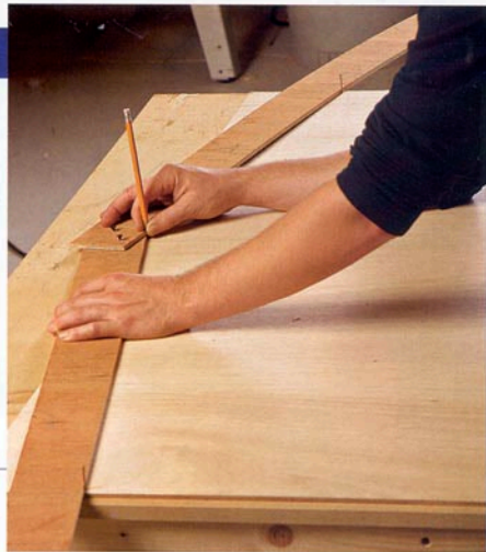
Arc jig. This simple jig allows you to draw a perfect arc of almost any size without having to calculate the radius.
