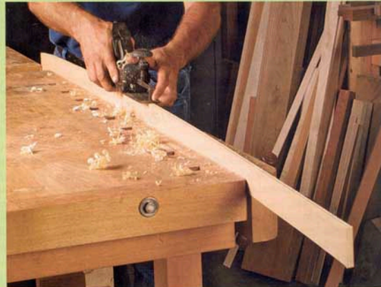
Plane a convex curve. With the sole of the compass plane set to the desired curve, make several passes, putting pressure on the nose of the plane until the curve in the workpiece is fair.
