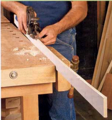
Plane a concave curve. Tune the sole to a slightly tighter inside radius than the curve to be planed and keep pressure on the nose with each pass.
