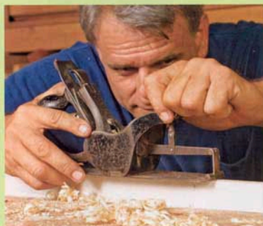
Adjust the curve of the sole. In addition to setting the blade, an adjustment knob on the compass plane changes the curve of the sole to a convex or a concave shape.
